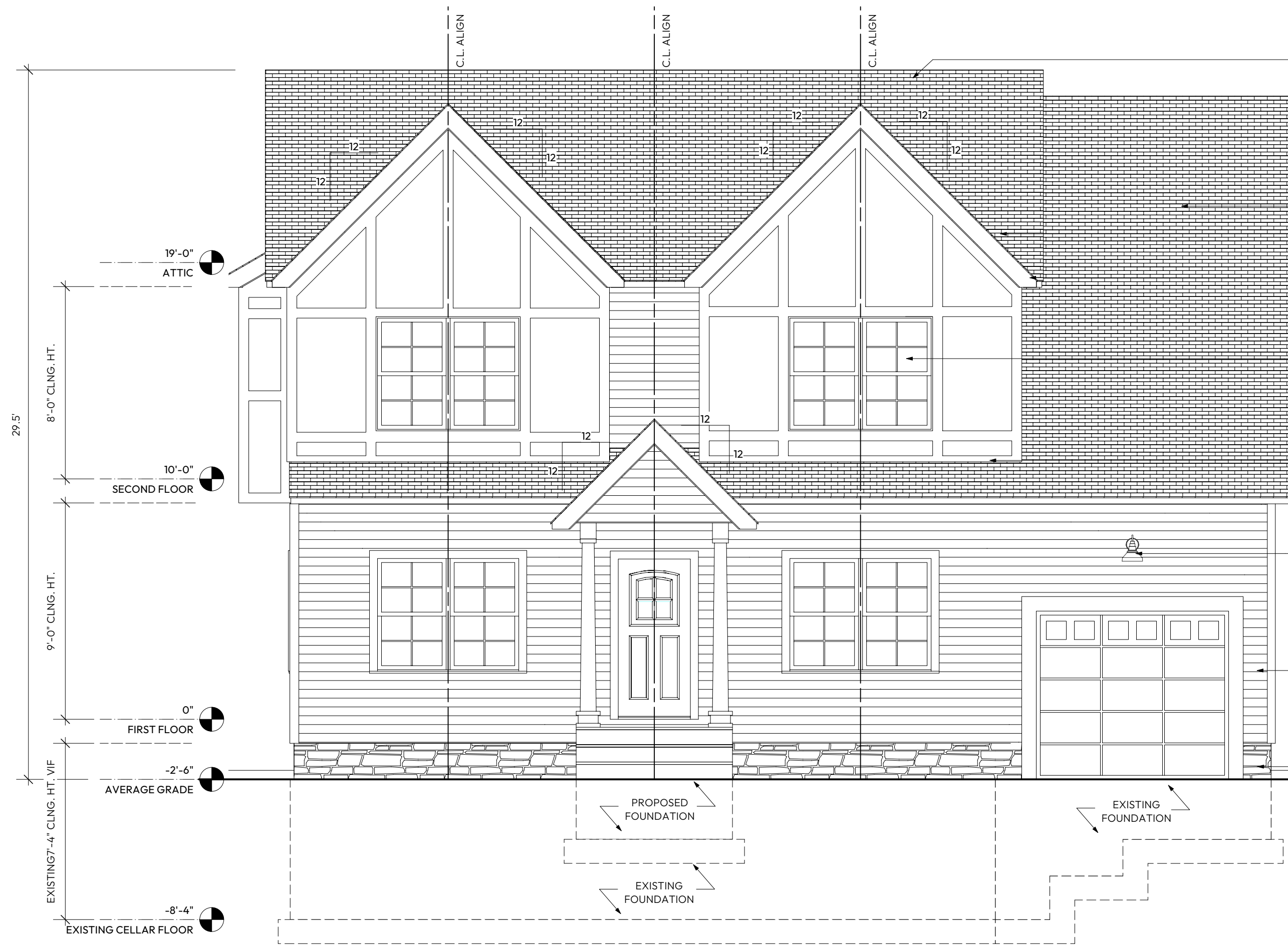
1 FRONT ELEVATION Scale: 1/4" = 1'-0"
